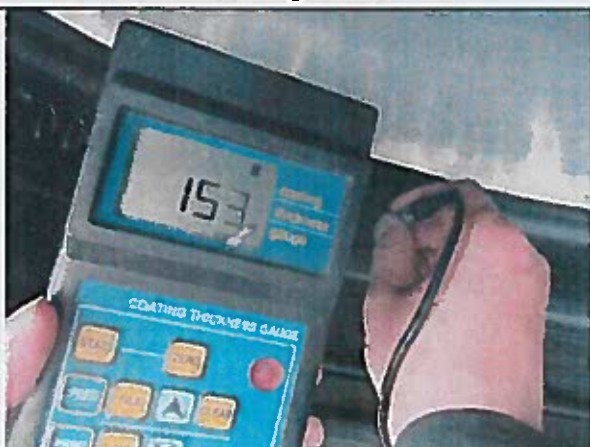
External coating thickness measuring
